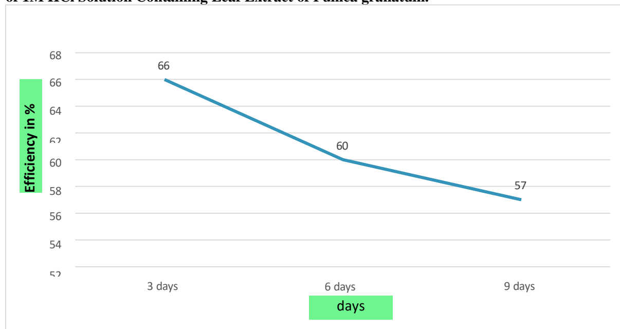
Figure 4: Shows the Efficiency vs. Time for Mild Steel in Uninhabited 1M HCl Solution and Inhibited of 1M HCl Solution Containing Leaf Extract of Punica granatum.
