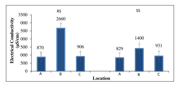
Electrical conductivity (EC) was highest in location B (2660  $\mu$ S/cm) and lowest in location A (870  $\mu$ S/cm). The mean value of electrical conductivity (EC) in both RS and SS effluent ranged from 829  $\pm$  6.8 – 2660  $\pm$  11.0  $\mu$ S/cm (*Figure 3*) in the study area. EC gives an idea of the amount of dissolved ions in the effluent (Yilmaz and Koc, 2014). Raw sewage (RS) had higher EC in all three sample areas
