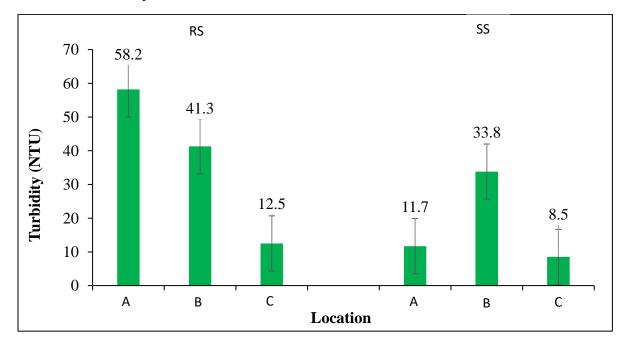
The results from *figure* 6 demonstrate that turbidity of effluent samples decreased along with locations
