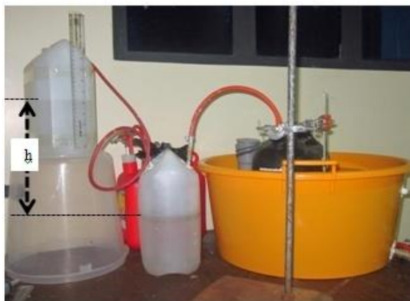
Figure 2: Setup showing the height ‘ h ’ that sustains high pressure in the biogas reservoir
