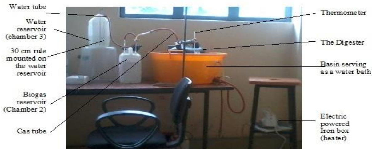
Figure 1: The setup of the actual laboratory-scale biogas digester designed and built in house by the author
