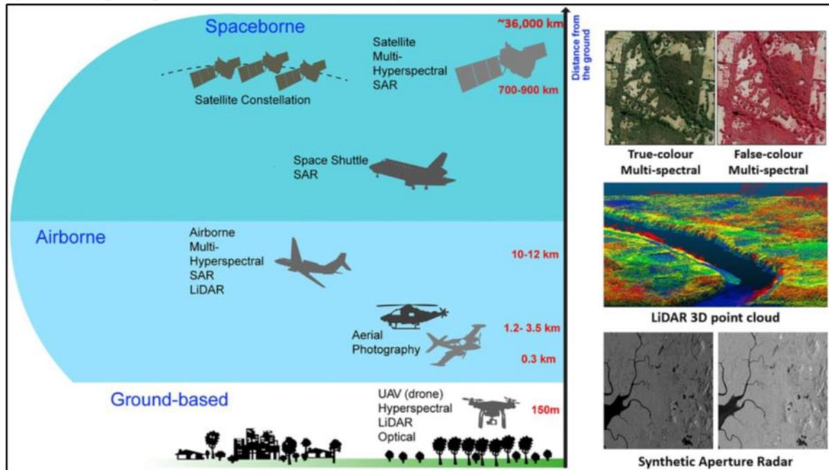
*Note: For each platform, the most often used sensors are shown on the left. (on the right) SAR data for the two polarizations via Sentinel 1 (bottom), LiDAR point cloud images of vegetation next to a river (middle), and true-colour digital aerial photography and fake color with NIR sensing (top).*
