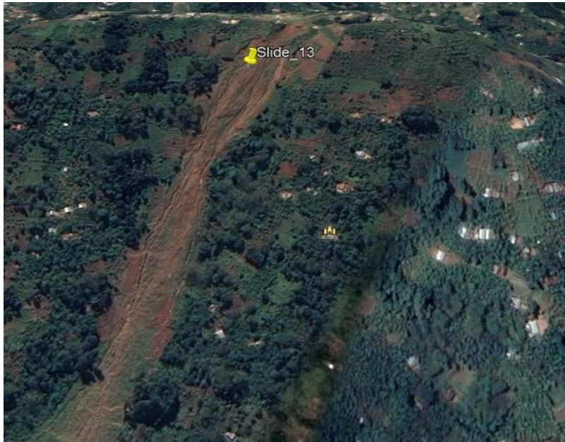
Figure 2: Landslide scar observed from Google Earth. Removal of vegetation as an indicator
