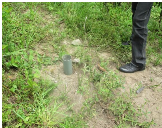
Figure 4: In situ Soil Permeability Test at the Mont-Amba site.
