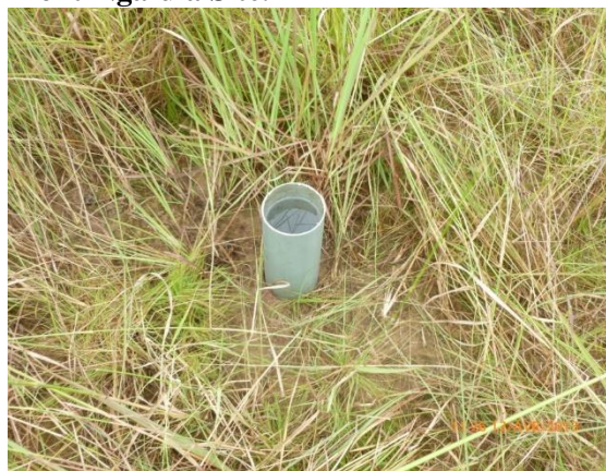
Figure 5: In situ Soil Permeability Test at the Mont-Ngafula Site.
