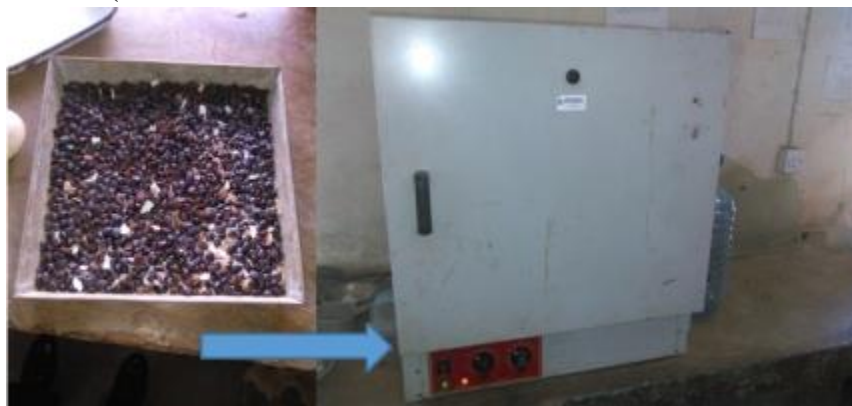
Plate 1: (Heat Treatment of Tamarind Seeds at 100°C to Remove Moisture Content)
