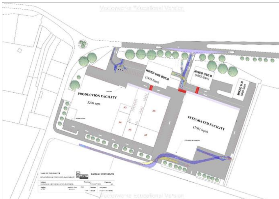
Figure 8: Truck Swept path analysis simulation using Autoturn Pro in BricsCAD
