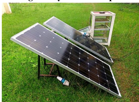
Plate 1: Set up of the experiment showing the dryer and solar panels Plate 2: Charge Controller and Deep Cycle Battery
