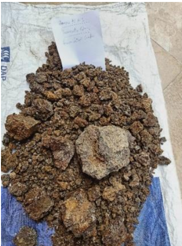
Plate 1: Sampling preparation of cinder gravel and blending material for testing
