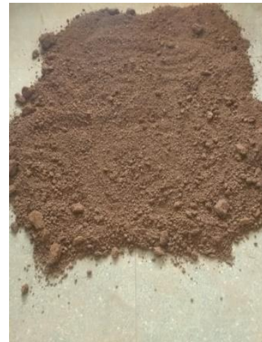
Plate 1: Sampling preparation of cinder gravel and blending material for testing
