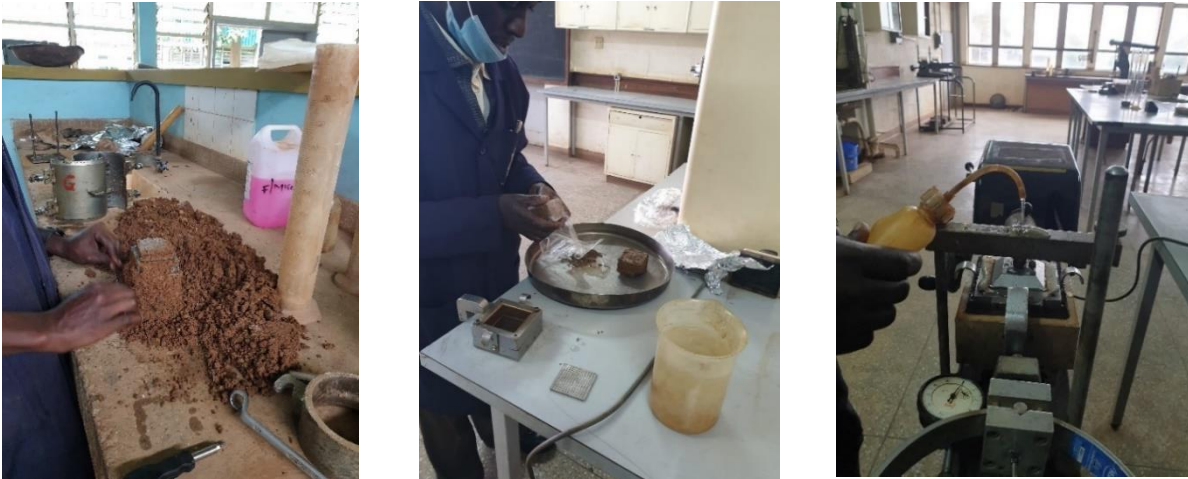
Trimming and extracting specimens from compacted samples extruded from the split mould Extracted specimen being covered with a cling film foil paper for 24 hours before testing The specimens were soaked for a few minutes prior to shear box testing
