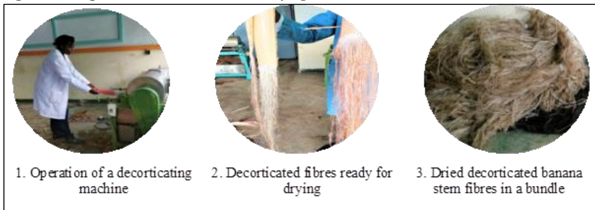
Figure 1: The process of decortication and drying of BS fibres
