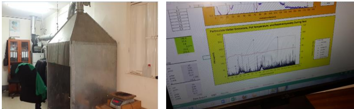
Figure 4: Left- Set up of LEM; R- Particulate matter emissions reading during WBT experiment
