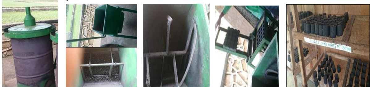
Figure 3: L-R- Carbonizer; Residue crashing machine; Mixer; Compressor and Drying racks used for the study
